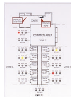
Typical purpose-built indicating boards: Left Fire fan indicator panel Right Network zone index
