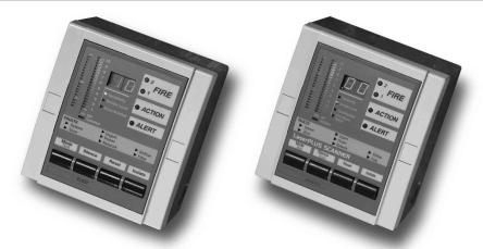
Display modules provide real-time indication of the status of an VESDA detector. They have a 20-segment vertical bar graph display, a 2 digit numeric display, an audible sounder, clear alarm and fault indicators. They also have 4 push button keys to control the detector and the mode of the display.
