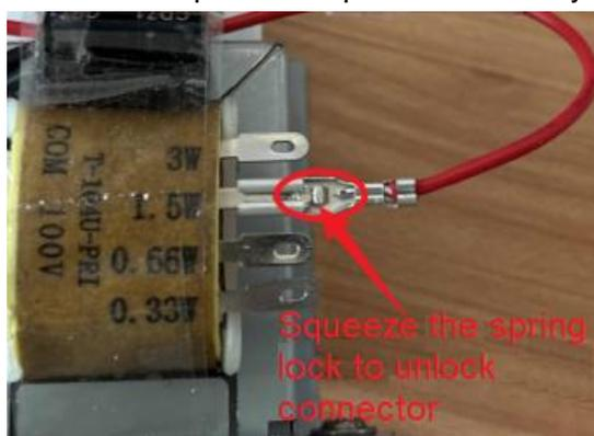
Gently pull the connector to unplug it and fit it to the desired tap.
