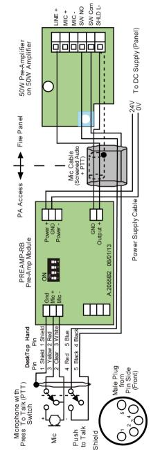
Failure to connect the microphone Shield may reduce the quality of the signal received by the 50W Amplifier Pre-amp. The shield must not be connected to panel Earth because Earth Leakage currents caused may impact the quality of the signal received. Note:
