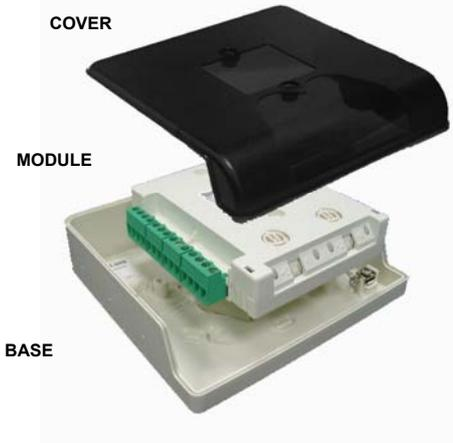
Surface Mount Box Base is affixed to mounting surface, and then the module and cover are screwed onto the base using the two screws supplied.
