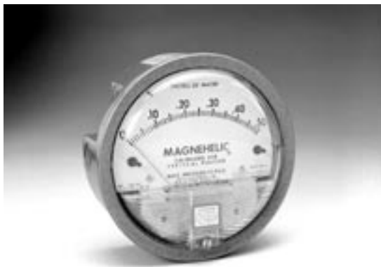
Figure 14: Magnehelic gauge for reading static pressures in air systems
